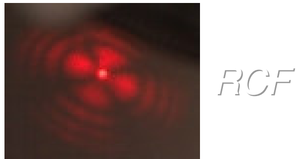
Figure. 4. Photography of the isogyre pattern observed with set-up. The dark cross and the concentric circles are clearly visible.
