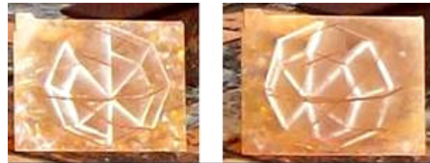
Figure 3. Stereoscopic pair from the 3D image of a polyhedron obtained at two different angles. The scratch hologram was laser engraved on a transparent acrylic piece. The image were obtained using sunlight illumination in reflection mode.
