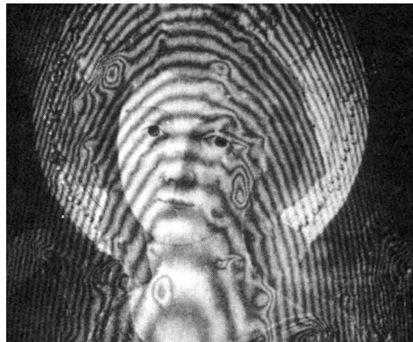
Figure 2. Holographic interferogram revealing paint-layer detachments.
