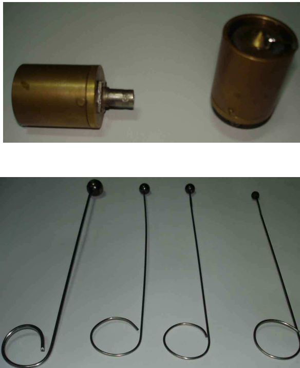
Figure 3: Photographs of the Pick up transducer and impactors.
