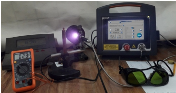
Figure 4. Experimental setup for the evaluation of the FISSEHighBeam10 . The multimeter, with a connected thermocouple, monitors the temperature.
