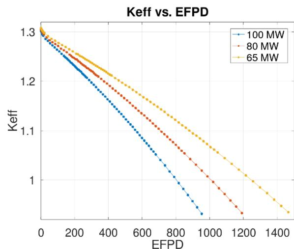
Figure 2.  $K_{eff}$  vs. EFPD for different values of core thermal power.
