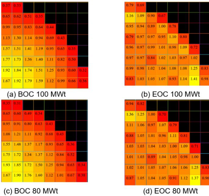
Figure 3. Radial power distributions at BOC and EOC for fuel cycles with difference power values.
