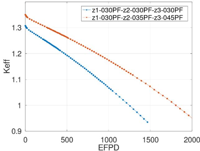
Figure 7. Keff vs. EFPD for different core compositions with three zones.
