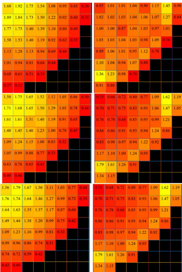
Figure 6. Radial power distributions at BOC and EOC for the different reactor core compositions. Up to down: a) Z1-0.30 and Z2-0.30 (BOC and EOC) b) Z1-0.30 and Z2-0.35 (BOC and EOC) c) Z1-0.35 and Z2-0.40 (BOC and EOC)
