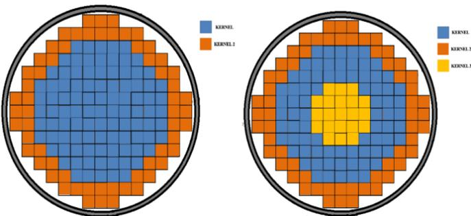
Figure 4. Fuel assemblies' layout for two and three zones core.
