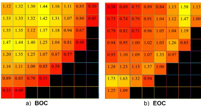
Figure 8. Radial power distribution at BOC and EOC for the core with three-zone composition, PF values of 0.30, 0.35 and 0.40 in the inner, middle, and outer zone respectively.
