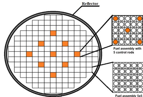
Figure 1. Scheme of the proposed reactor core with 157 fuel assemblies.
