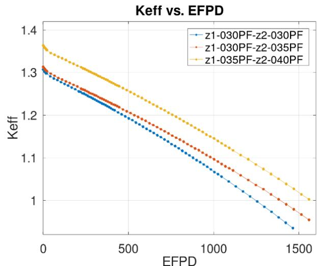
Figure 5. Keff vs. EFPD for different core compositions with two zones.
