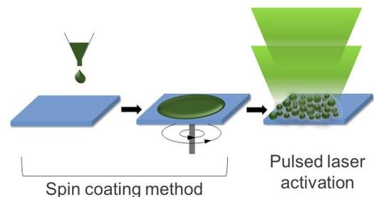
Figure 2. Diagram of the obtaining of the ZnO seeds layer using the spin-coating method and pointing a pulsed laser on the sample.
